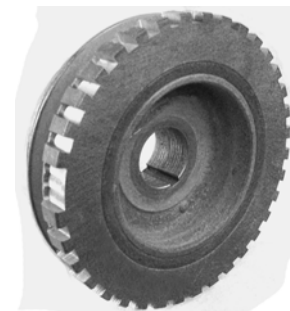
Harmonically balanced pulley - machined into trigger wheel
