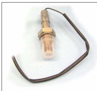
Typical single-wire narrow band oxygen sensor
