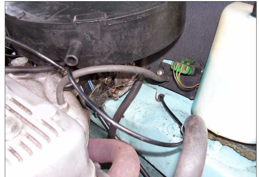
MAP sensor installed in Mini, with vacuum pipe connected to inlet manifold take-off
